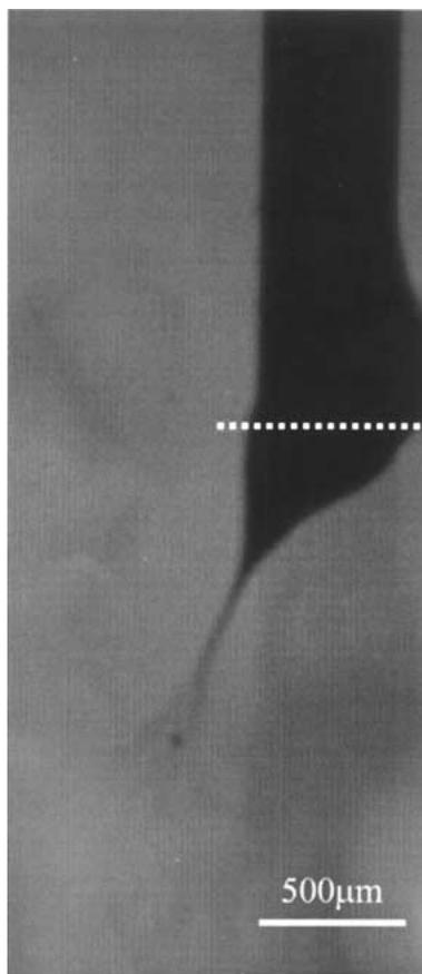
Figure 2 Electrospinning of the nHA suspension as captured by a MotionBlitz high-speed camera (Weinberger AG, Dietikon, Switzerland). The dotted line represents the exit of the needle.
