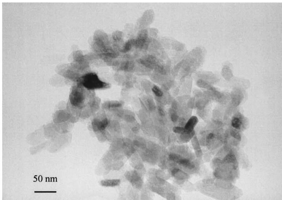
Figure 4 Transmission electron micrograph of typical nHA relic produced by electro spraying.
