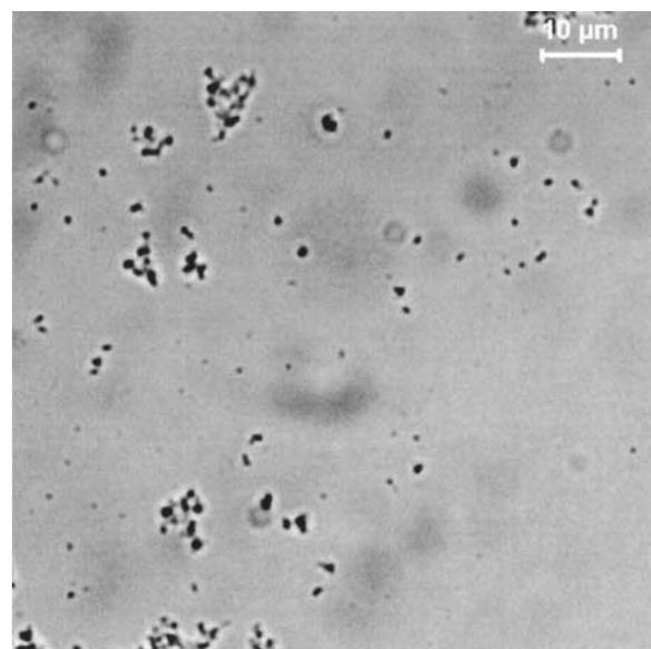
Figure 3 Optical micrograph of electrospayed nHA relics on a glass slide.
