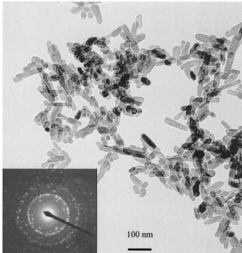
Figure 1 Transmission electron micrograph and selected area diffraction of nHA particles.
